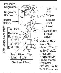
\* A CSA design-certified equipment shutoff valve with 1/8" NPT tap is an acceptable alternative to test gauge connection. Purchase the optional CSA design-certified equipment shutoff valve from your dealer. See *Accessories*, page 33.
